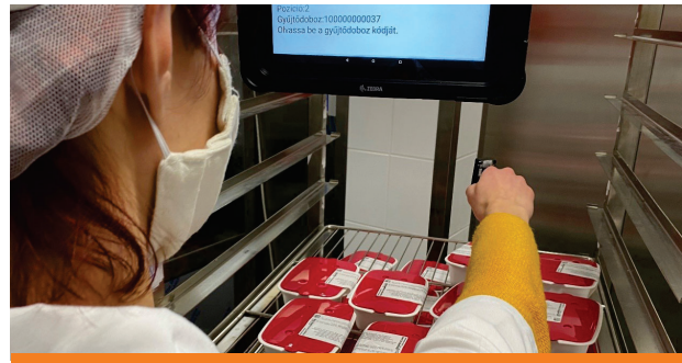
Preparing food for institutional delivery, the worker reads the GS1 DataMatrix barcode on the label for transportation in the heat storage to the institution.
